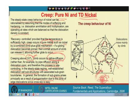
So, the mechanism mostly involved with the desired steady state creep at a given stress and at a given temperature level. So, for very common purposes of superalloy development, we apply actually 170 or 172 MPa stress and the first generation, second generation, third generation, or fourth generation and this generation of several superalloys has been developed in terms of a higher stress and higher creep life means time to rupture.
