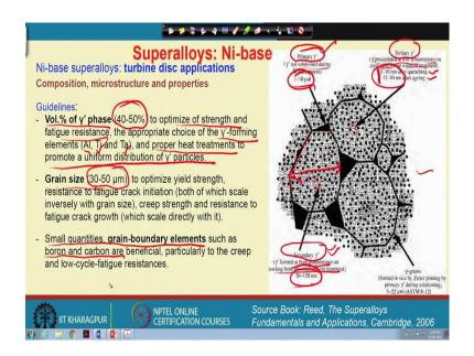
So, design consideration includes that the volume fraction of the  $\gamma'$  phase should be 40 to 50%.
