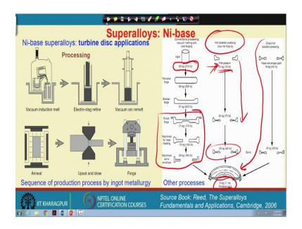
Now, for a disk application, we should have a look at the different processing technique. To make a disk, we have to go for some particular shape which appear like this is a section. So, we start with Vacuum Induction melting then we go for some Electro slag refining process. So, that we remove some of the slag and make a purer alloy then we go for some vacuum arc re-melting so that any kind of dissolved gases to be came out after that we go for some heat treatment.
