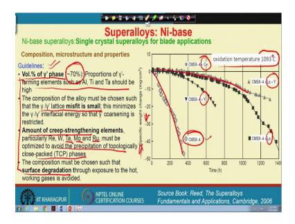
Now, if you think about some of the composition microstructure and properties of these superalloys the volume fraction of  $\gamma$ -phase should be higher like 70 % and the portion of  $\gamma'$  forming element that should be high. So, there are some design consideration. So, I am just talking about the design consideration. However, the misfit should be small. So, that we will get effective strengthening
