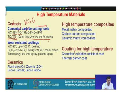
So, for tool material the very important cutting tool material are the cemented carbides, because carbide gives the very high strength and we have 5 to 10 % metal matrix that basically give advantage of a larger toughness; so, this name is itself is Cermet. So, the Cermet name came because of the ceramic and metal.
