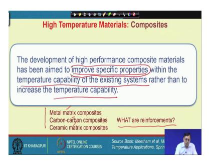
Now, if we think about composites, composites are developed not to enhance the limit of the temperature. So, the development of these high performance composite material is aimed to improve some specific properties, within the temperature capability of the existing system rather than the temperature capability. So, this is very important aspect when we really need to develop a composite.
