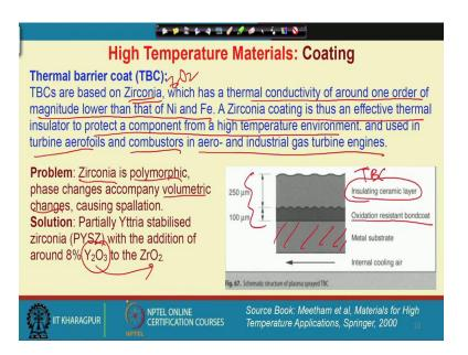
Now there are another two type of coating; one is oxidation resistance coating and another is thermal barrier coat. Thermal barrier coat basically contains zirconia; zirconia is zirconium dioxide, which has a thermal conductivity, which is one order magnitude lower than any of the nickel and iron.
