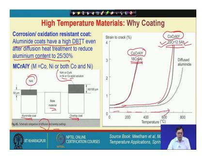
So, let us see one of the example of such corrosion resistance coat, where you can see here the amount of chromium aluminium has been changed in this particular coating that I just told you. And with the operating temperature, by changing the composition, this is the strain that require cracking. So, it improves. So, we can use or change the composition for a better service life.
