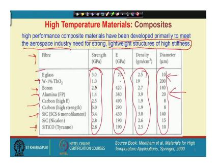
So, here for the composite, let us have a look at these different fibres that we can employ. So, the basic purpose of using this composite is aimed for developing primarily to meet the requirement of the aerospace industry, for very strong lightweight structure with very high stiffness.
