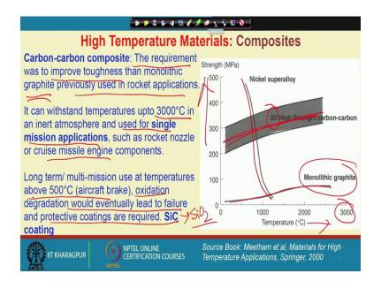
Now, the other composites are like the carbon-carbon composites; and you may recall that carbon-carbon composites could survive at much higher temperature than the any metal matrix composite because carbon itself is a high temperature material, but carbon appear as a graphite, where graphite oxidises into carbon dioxide and leaves the material.
