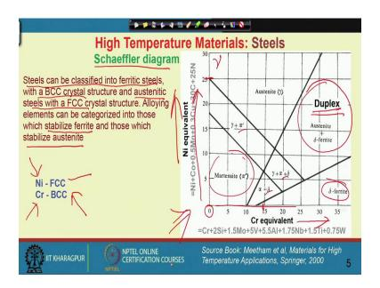
So therefore, the steels also classified into ferritic steel with BCC structure or austenitic steel with FCC crystal structure, it is very clear. Now the alloying element also can be categorised as a ferrite stabilizer or austenite stabilizer. However, to understand this, we need the help of a diagram which you already have learned in a physical metallurgy classes, which is called as Schaeffer diagram.
