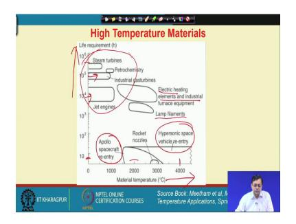
Here, we have plotted the demanded life of a component with the temperature or operating temperature of a material, you can see that around  $10^6$  hour required for using a steam turbine. Because repetitive times long time duration the steam turbine has to be used, very similar like petrochemical industries or industrial turbines and relatively lower life is expected in a jet engine.
