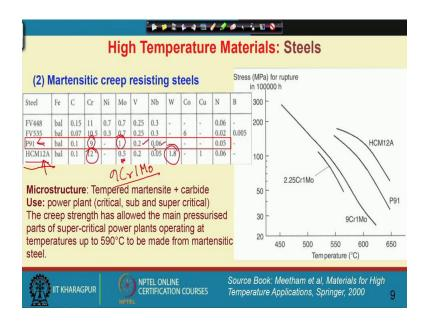
Now, let us talk about the martensitic creep resistance steel, so the name itself said again that they contain martensite microstructure. And now what is the operating condition of the steel yes it should be a minimum something like 500 or 600 °C, so the martensite phase should be stabilized, but is it possible or not that is another question, but let us look at what is desired out of the steel.
