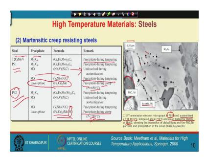
So, the other purpose that we must discuss that what are the precipitate expected from this P91 or this advanced steels. So if you kindly have a look at the 12CrMoV here there are  $M_{23}C_6$  carbide and this is a precipitation hardening alloy, due to tempering of the martensite. Whereas, P91 has these Laves phase, which has been precipitated during creep
