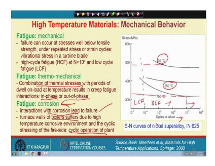
And here let say you can see that a lower temperature we can use a higher stress, higher as at higher temperature we have to go for low stress in order to ensure that the material will survive at higher cycle.
