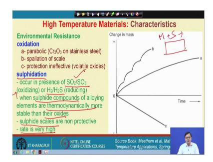
And they basically react with the sulphur. So, metal react with the sulphur to form sulphide compounds.
