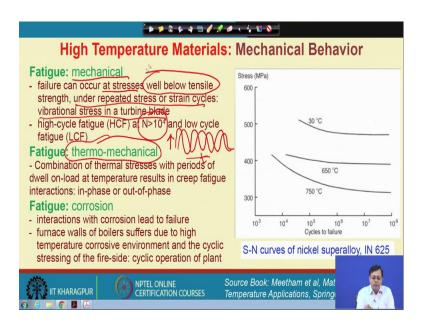
However, we can also think about the fatigue behaviour of materials because fatigue is important aspect of another mechanical properties. So, this fatigue could be mechanical fatigue, means the failure can occur at a stress well below the tensile strength level. And under repetitive cycle or repetitive stress or strain cycle like a vibrational stresses that occur in a turbine blade. The situation may be very different.
