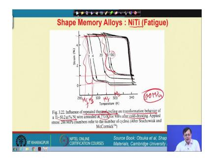
Now, similar effect we can see in case of a thermal fatigue, means, if I keep on increasing and decreasing the temperature what will be the effect, this is very interesting phenomena. Please have a look here, this is a repetitive thermal cycling on the transformation temperature and behaviour of a titanium-nickel alloy, which has been annealed at 773
