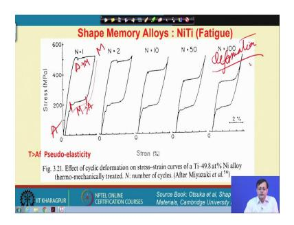
And here austenite transform into martensite the same thing is here, so, this is a very interesting phenomena. However, this is a deformation induced or cyclic deformation induced fatigue on the shape memory effect on the pseudo-elasticity.
