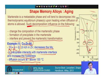
So, let us start with first the aging phenomena in case of a copper base or non-ferrous alloy. So, what we really mean by aging, martensite is a metastable phase, there is no doubt about it, because it is a diffusion-less phase transformation, martensitically transform product from the austenite phase. And it will always tend to decompose once into a thermodynamic equilibrium phase upon heating, once we have allowed some activation energy for diffusion to occur.
