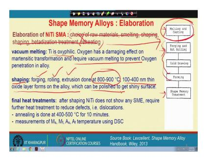
Now, let us discuss about another system very important non-ferrous shape memory alloy system. In that case, actually we will talk about nickel-titanium alloy. In case of nickel-titanium alloy, the choice of raw materials melting or shaping, betadization and reheating, are not at all required like in case of a copper-base shape memory alloy. So, these system we do not need at all.
