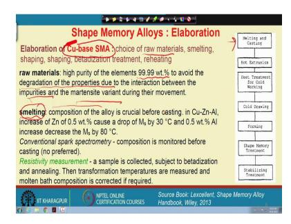
Now, the second part of today's talk is on the elaboration, elaboration means to achieve a final product from the initial alloy, from the alloy making. In this particular case, let us say, if I take a copper base alloy copper base system, here in this particular case, the elaboration technique contain let us say the choice of the raw materials smelting, shaping and let us say the betadization treatment.
