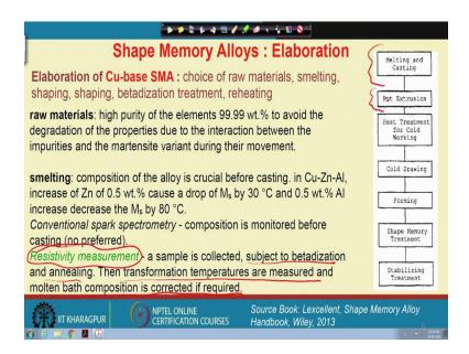
However, conventional spark spectrometry does not give you very accurate result. In that particular case, what we do, we simply collect a liquid alloy, and then we solidify it by casting which is subjected to betadization. I will come to betadization treatment what is the meaning of betadization and annealing.
