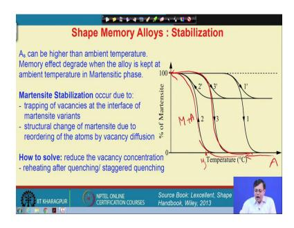
Now again I let say cool from the austenite, and then during cooling here at this temperature, martensite start temperature, the transformation begin, so I have martensite plus austenite in this region. And then all the austenite transform into martensite. Now, if we reheat it, so this is like a cycling, then in the third sequence, it will go in this way; there is little effect on that.
