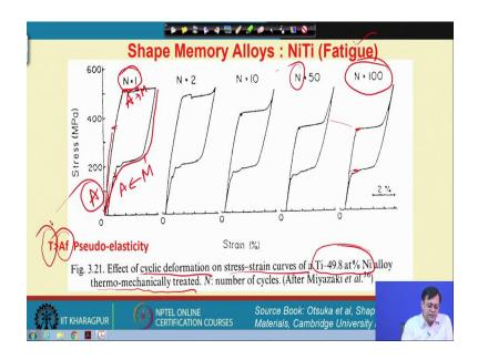
How the curve basically looks like means that. I start with austenite and here, the austenite started transforming into martensite. If I unload it, then again it goes back, because here martensite will transform into austenite.
