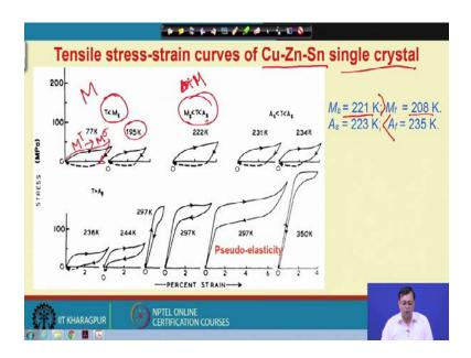
Now, let us consider one of such very interesting tensile stress strain curve of a copperzinc-tin single crystal which is also well known as a shape memory alloy. And this is the single crystal, please consider the martensite start temperature is 221 K and martensite finish is 208 K which is lower than  $M_S$  as expected and austenite start is basically 223 K and austenite finish is 235 K.
