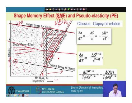
If we increase stress, then martensite start temperature will increase. Please have a look at this particular diagram and this particular aspect because there are lot of thing to discuss here. And if that is the condition mean stress increases the martensitic start temperature increases and the shape memory effect means deformation should be given to achieve shape memory effect should be lower than the  $M_s$ .
