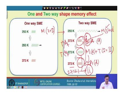
In such a condition, I will have large plastic strain. In this condition, what we have? We have martensite, martensite means I type of twin and type-II twin here and if I strain too much, then let us say I have martensite with twin; however, this twin plus some dislocation will form because I have strained it too much,. And so, under such condition, if I heat it up, then I will have austenite. So, here temperature is greater than austenite finish.
