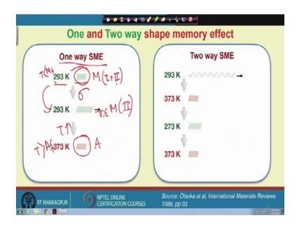
So, far, we have discussed one way shape memory effect; means let us say a martensitic spring is kept at 293 K, this temperature is well below the martensite finish temperature.
