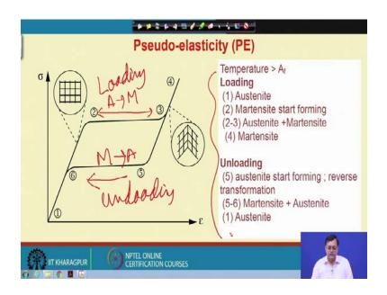
And we have already looked at that from 2 to 3 in between these what austenite transform to martensite and here during unloading cycle, this is the loading cycle and this is the unloading cycle.
