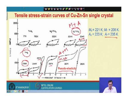
In that case actually, we see that the recovery has increased. This means, some part of the austenite must have transformed to martensite during deformation itself. Now, we increase the temperature further to 236 K, which is above austenite finish. So, here we see that the recovery of that strain has increased and if we keep on increasing, we can see from here itself, 297 K we can get back the 100 % strain.
