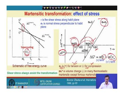
Because I had told you that, we need some excess super cooling in order to form a martensite. And this particular  $G_m$  or the  $\Delta G$  for nucleation of the martensite require some supercooling.
