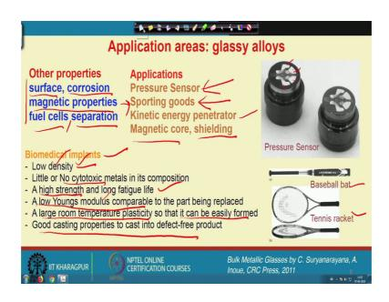
So, in both the cases we have shown that there is a large plasticity we can get out of such microstructure. And now let us come to some of the very critical application the glassy alloys are always at the top in competition with the conventional crystalline alloys. So, there is no other material which can show such kind of application areas.
