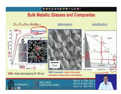
And definitely the shear bands at somehow linked with the thickness of the sample and so on. However, when we talk about bulk metallic glasses very bulk the separation distance between 2 shear bands is in the order of something like 10 to 50 or even 100 micrometer. So, if we take such a bulk metallic glass and compress it we will get a engineering stress strain diagram in that particular case we will get only the elastic deformation this is just a schematic deformation elastic deformation plot.
