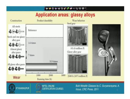
Now, that is another very good area where there is no competition with the glassy alloys. It is basically in terms of wear, wear and tear of glassy phases are very very low. So, let us say for using any or making any gear we usually use some hardened steels ok. So, in that case definitely these gears could be very large to a micro meter size and since glassy alloys or monolithic glassy alloys are isotropic in nature not like crystalline materials.
