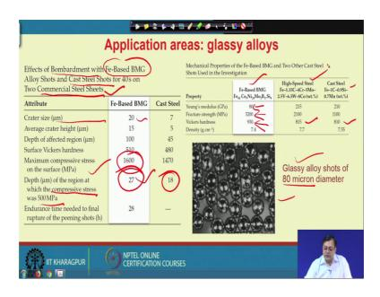
Now, there are another very large application areas we secondary process material the example is shot peening ok. We bombard sand particle on the surface of a metal in order to change a or in order to introduce some compressive residual stress and better surface finish or let us say the better surface for a good fatigue life. So, in those particular aspect we can use actually the glassy balls ok.
