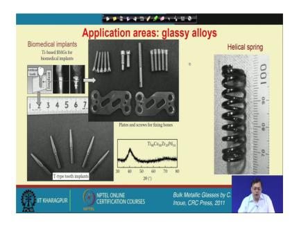
So, this screws are and the plates are made out of this bulk glasses or let us say some sort of t type of tooth implant could be made out of these titanium base glasses. So, that we can replace the titanium aluminium vanadium or let us say some of the helical spring which are very common mentionally used it has a very very high elastic limit and resilience. So, several times we can use the same helical springs means the durability will increase.
