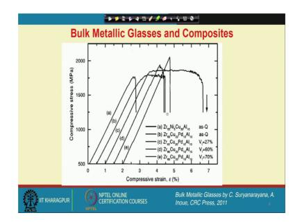
Now, along this direction as I said that people have also tried to incorporate some nano crystalline particles into a glassy matrix and you can see that the curve A which is from a zirconium nickel copper and aluminium very common glass, which is in the as quenched state or let us say a, b, b here is the is the palladium base glass, which itself show some plastic strain in the as quenched state.
