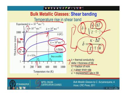
So, one has to has to estimate that a since it is a adiabatic process, the formation of shear band occur very very rapidly or strain is localized those event occur very very rapidly and so, in the order of some millisecond and so on.
