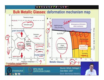
So, similarly here also this  $\tau/\mu$  is also give the same type of relation that is the shear stress by G, because G and tau are the same. So, instead of a calling it as a normalized stress, we can also call is something like it is equivalent to some sort of critical strain in the in the material and in case of metallic glass this deformation map has been designed because the T g is important here
