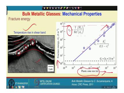
So, definitely the question will appear that these shear bands whether how temperature are related with formation of this shear bands, since the deformation and strain is localized whether there is any adiabatic heating. And one should look at the fracture energy of these bulk glassy solids and also the plastic zone size; People have measured all these values and observed that the plastic zone size definitely is higher in case of a higher a fracture energy which is also very very high.
