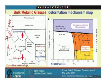
So, all these mechanism that I had discussed in this local deformation homogeneous inhomogeneous flow, recently it has been a summarized and a people come out with some deformation mechanism map. And this deformation mechanism map is also available in case of a crystalline metals and alloys. So, I think we can simply first have a look at the deformation mechanism that is available or existing for crystalline metals and alloy and then we can simply try to compare in case of a glass.
