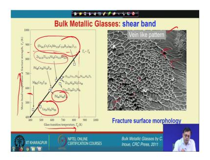
And therefore, when we study the fracture surfaces of a metallic glass, usually we observe such kind of vein like pattern. Even though they have some similarities of melting all let us say like separation of breeze ok. So, those kind of feature can be observed.
