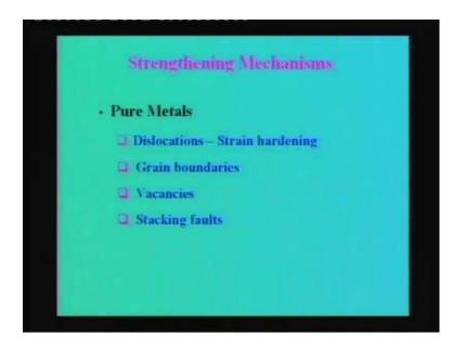
So, people have a shown that one way to achieve high strength, at the same time high toughness is to make the grain size final. So, if you look at pure metals, what are all the different strengthening mechanisms in pure metals. As we can see, one fast and foremost is that we know there are dislocations in the material.
