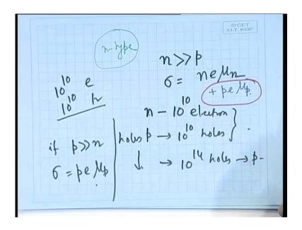
Suppose there is a material you have doped it n-type there is a material you have doped it n-type, this n-type material has both electrons and holes. You can tell me sir from where the holes are coming because one thing is sure that we have started with intrinsic materials. So, in intrinsic materials there are electrons as well as holes or say you have formed one p-n junction.
