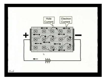
And, here if you apply a current or a say you apply a voltage; that means, electric field. Here see you have applied a voltage, and this is the positive terminal of the battery, this is the negative terminal of the battery. So, there will be a flow of current from where in the opposite direction, the electron moves in the opposite direction. So, that is very important thing that you see that the electrons move in this direction. So, the current will
