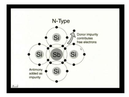
So, here who is the host lattice? Silicon is the host lattice, and dopant is phosphorous. Here the picture is more clear, the same picture. Here the picture is clearer you see that 1, 2, 3, 4, 5, 6, 7, 8 they form the bonding and the 5 th electrons is away. So, basically you need for 4 silicon atoms you need one antimony atom. For 4 silicon atoms you need one antimony atom or one phosphorous atom. Then after doping what will happen?
