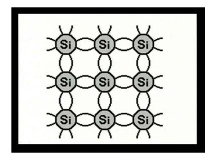
And, if you look at the picture, you see that this is the 2 dimensional diagram of silicon atomic arrangement inside the lattice. What is the valence of silicon? 4.
