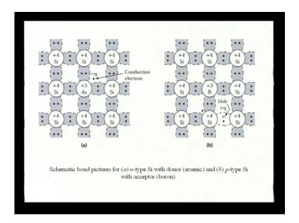
So, this is the schematic bond pictures for n-type silicon here we have used the arsenic as a donor and here the boron and already we have shown already we have seen that this is the free electron or this is the hole which is to be filled by the adjacent electron. So, when this electron moves here there will be a hole created here then this electron will move here to fill that hole. So, there will be a hole transport in the material for P-type semiconductor.
