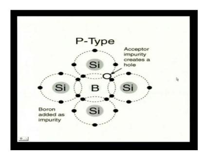
This picture will show you that phenomenon. You see that when silicon is doped with boron; boron has 3 electrons, silicon has 4 electrons. You have 7 electrons in this system. You need how many electrons?
