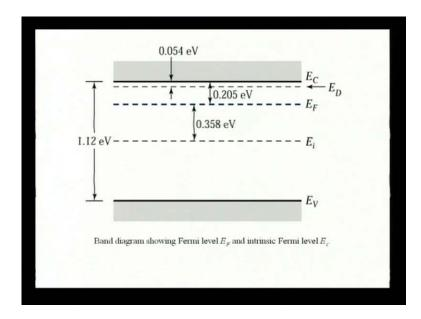
So, these things we have discussed. Now, another important thing is the intrinsic level E i, E i is the intrinsic level. What is intrinsic level? Intrinsic level is an imaginary electron state or imaginary level inside the band gap which is almost half away from the bottom of the conduction band or the top of the valence band. And, it is applicable for intrinsic materials only where the number of electrons and number of holes are equal.
