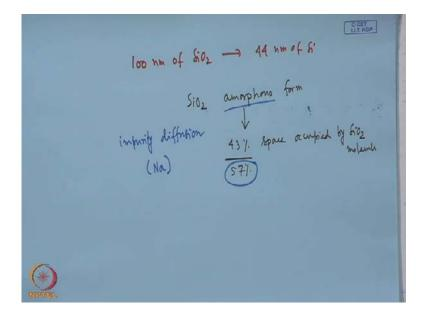
So ,in S i O 2 amorphous form, you see that there is 43 percent space occupied by S i O 2 molecules, so almost 57 percent is void and this 57 percent void space. This 57 percent void space has some bad effect, in the sense that there can be impurity diffusion as it is amorphous in nature. So, impurity diffusion will be there particularly sodium and
