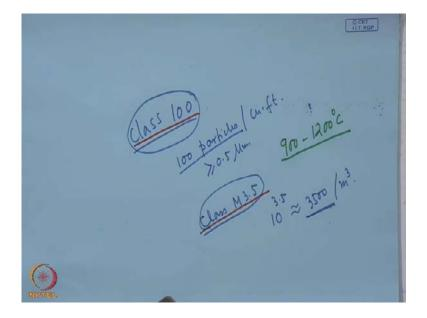
So, everything will be settled by the microprocessor control and in this case you see that apart from these gas flow sequence and automatic insertion and unloading of wafers temperature you have to increase, because the temperature required in this case is normally 900 to 1200 degree centigrade, this is the temperature required for the oxidation.
