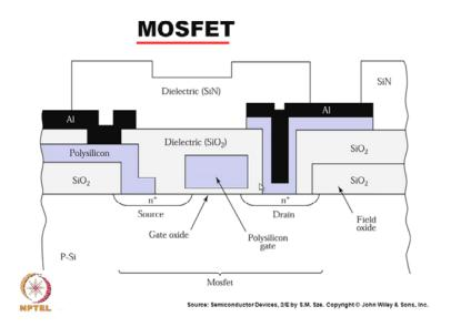
Today's topic of discussion is the oxidation, and you can see from this view graph that there are different types of layers that we use for making a discrete device or an i c, they are say gate oxide then there can be field oxide, the poly silicon gate or some dielectrics and finally the metal layers.
