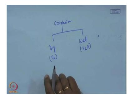
There can be two type of oxidation; one is the dry oxidation and the second one is the wet oxidation, so depending on the source of oxygen available in the oxidation process. For dry oxygen generally oxygen high purity oxygen gas is used whereas, for wet oxidation high purity water vapour or steam is used. So, depending on the nature of the source that you use for an oxidation process, it can be termed as a dry or wet oxidation.
