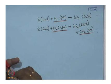
Now, with this value, let us consider that how this S i O 2 layer is grown? In this case, the S i O 2 layer is grown, suppose you have S i which is nothing but the solid it reacts
