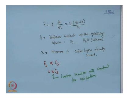
Now, with this idea, so let us consider that F 1 is the flux, which we can say that it is equals to D and d c by d x, where D is the diffusion constant of the oxidizing species that means; oxidizing species may be, it can be oxygen molecules or water vapour. That means, steam, now this is equals to, we can write D C 0 minus C s by x as you can find,
