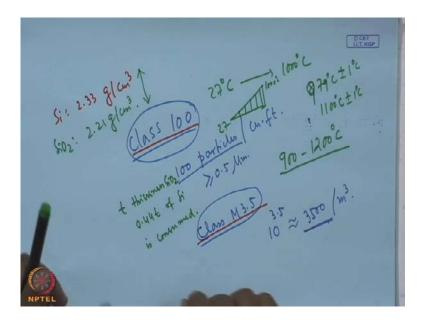
The corresponding values; that means, the molecular weight of silicon dioxide is given as 60.08 gram per mole and 2.21 gram per centimeter cube is the density of S i O 2. So obviously, you see that the density of S i O 2 is less than the density of Si, Si density is 2.33 gram per centimeter cube, whereas for S i O 2 it is 2.21 gram per centimeter cube so; obviously, if you compare with the silicon the porosity is larger in case of S i O 2.
