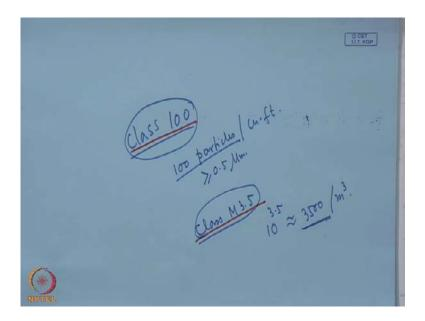
So, this is known as the class 100 clean room or in metric system, you see that it is a a logarithm of the maximum allowable number of particles and the particle size is same in this case also, it is 0.5 micron and larger per cubic meter. So, in metric system, it is per cubic meter and in English system it is per cubic feet. Now, what is a class M 3.5? M stands for metric, 3.5 it it means 10 to the power 3.5 or at the most 3500 particles per cubic meter per cubic meter it is allowed.
