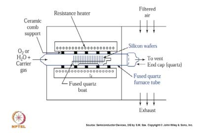
Now, this is a typical oxidation reactor, you see that in oxidation reactor, there are many components available in the oxidation reactor; one is the resistance heater which is used to heat the substrates, there is a quartz boat on which the silicon wafers are placed vertically, you can find that a large number of silicon wafers are kept here in the vertically in a vertical position on the quartz boat, and oxygen or H 2 O is passed through the quartz reactor.
