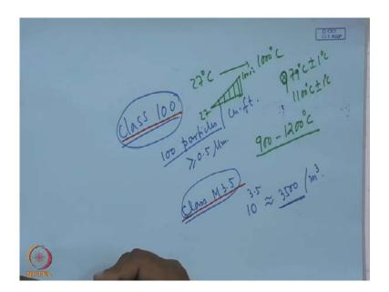
So, from room temperature say your room temperature is 27 degree centigrade, from 27 degree centigrade to say 1000 degree centigrade, we have to ramp the temperature very slowly. So that you can have here from 27 to 1000 degree centigrade, you can have, you can avoid the warping of the wafers, and to maintain the oxidation temperature within plus minus 1 degree centigrade.
