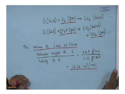
So, let us calculate say say the volume of 1 mole of silicon, volume of 1 mole of silicon if we write then you have to write that molecular weight of silicon by the density of silicon. Now, what is the molecular weight of silicon it is given, 28.9 gram per mole, you
