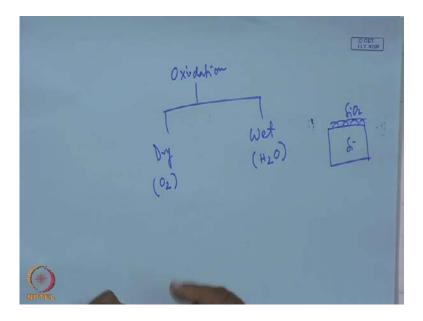
And you know that if you keep a silicon substrate open in normal laboratory atmosphere, we will find that some dangling bonds are formed on the top are taking the arial oxygen and it is very prone to oxides. So, a large number of interface traps will be formed in the the surface state density will be quite high, because of such dangling bonds.
