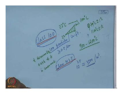
Now, it is very interesting to have the kinetics of growth, because you see that, when S I 2 is grown on a silicon, silicon is consumed and we shall see that if you want t thickness of the oxide film, t thickness of S i O 2, if you need, so 0.44 t of silicon is consumed. So, that is very important thing and if we discuss the kinetics of growth of silicon oxide, you will find that this silicon-silicon dioxide interface moves into the silicon during
