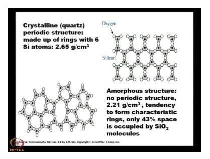
So, depending on the oxygen bridges, the crystalline or the amorphous structure is formed. Here you see that when this oxygen bridge is there and forms a ring, it is a ring like structure made up of 6 silicon atoms. This is 1 silicon atom, 1, 2, 3, 4, 5 and 6. So, 6 silicon atoms are there, if you consider here there is also 6 silicon atoms, so they formed a periodic structure. This periodic structure it has a it has density of 2.65 gram per centimeter cube.
