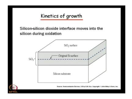
So, more and more silicon is consumed for the for the formation of SiO2 and one example that you can and try to solve if a silicon dioxide layer of thickness x is grown by thermal oxidation. What is the thickness of silicon being consumed? So, if it is x, then how much thermal oxidation and will be the silicon dioxide if a silicon dioxide layer of thickness x is grown by thermal oxidation?
