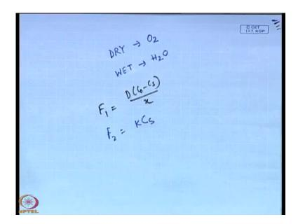
So, what we find that first this F 1 which we can write as d of C 0 minus C s by x and F 2 which we can write as k into C s. This C s is the concentration at the surface of the silicon. This is the concentration of the surface of the silicon then what is k? k is a surface reaction rate constant for oxidation. At the steady state this F 1 and F 2 will be equal and at the steady state this F 1 equals to F 2 equals to F.
