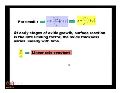
So, at early stages of oxide growth, surface reaction is the rate limiting factor. At early stages of oxide growth surface reaction is the rate limiting factor the oxide thickness varies linearly with time and this B by A is known as the linear rate constant. So, we shall arrive at two types of rate constant; one is the linear rate constant and another is that we shall discuss now it is for large T, when we shall find that this will vary as the parabolic nature.
