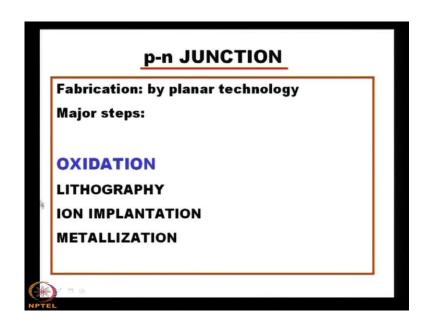
We can see that oxidation is the first one with lithography ion implantation metallization etcetera and this oxidation step very good quality gate oxide is required. Otherwise what will happen the leakage current will increase like anything, and because the leakage current increased and the interface states will be more in case of the leakage. So, gate oxide must have good electrical property and this electrical property can be achieved if we use the oxide grown by the dry oxygen method.
