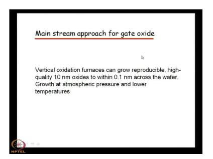
So, main stream approach for gate oxide is that one can use the vertical oxidation furnaces I have shown you the oxidation furnaces this is the oxidation furnace that we have discussed earlier. It is a horizontal type of thing and you see that here on the silicon wafers are placed on the fused quartz boat a large number of silicon wafers.
