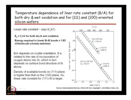
And here the parabolic rate constant or the linear rate constant we shall now, now see the variation of the temperature dependence or the temperature dependence of linear rate constant for two cases; one is when the wafer is 111 oriented or 100 oriented.
