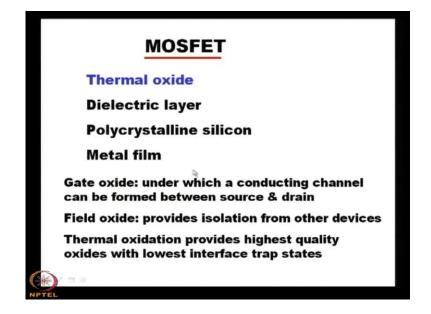
Then field oxide it is provides isolation from other devices and this two oxides are formed mainly by the thermal oxide, next day we shall discuss the dielectric layers or other polycrystalline silicon and metal film.
