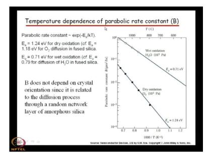
And this is the temperature dependence of parabolic rate constant parabolic rate constant B and quickly we can see that what is B? B is twice d C 0 by C 1, this d is the diffusivity or the diffusion constant, C 1 what are what are C 0 and C 1. C 1 is the value for for dry oxidation this is the number of molecules of the oxidizing species in a unit volume and C 0 is the oxidizing species at the surface. So, C 0 and C 1 we understand and from that we can know what is B the parabolic rate constant?
