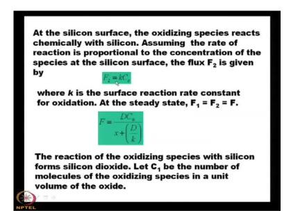
At the silicon surface the oxidizing species reacts chemically with silicon, assuming the rate of reaction is proportional to the concentration of the species at the silicon surface the flux F 2 in given by F 2 equals to k into C s.
