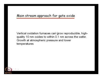
So, if you have a wafer say of 6 inch and the growth can be oxide layers can be of say 10 nanometer plus minus 0.1 nanometer plus minus 0.1 nanometer. So, that is very, very precise and this 10 nanometer is nothing but where we have we have seen that it can be it is it is used in case of the gate oxide in moss technology, and also the growth at atmospheric pressure and at lower temperatures.
