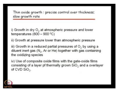
Another important thing from from this from this studies is that thin oxide growth thin oxide to grow précised control and to make the precise control over thickness slow growth rate is important slow growth rate is important where one can precisely control the thickness, because one can see that in process technology when we talk about the oxidation that this is the oxidation it is one of the process steps by planar technology.
