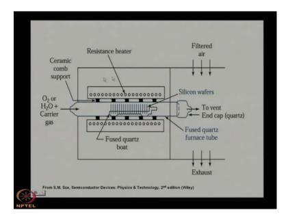
The whole thing means the first thing is that we have to load the silicon wafers inside the oxidation chamber another important thing is the enhancement of the temperature raising the
