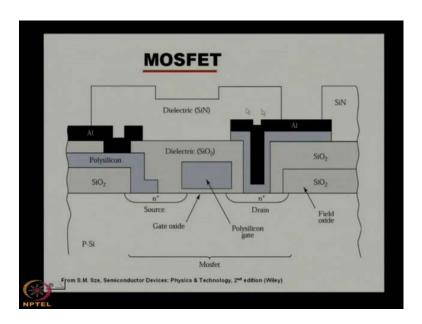
If you take another example of the MOSFET, you will find that this in MOSFET there are many kinds of dielectric poly silicon and oxide films like this gate oxide poly silicon gate field oxide dielectric like silicon nitride then Si O 2.
