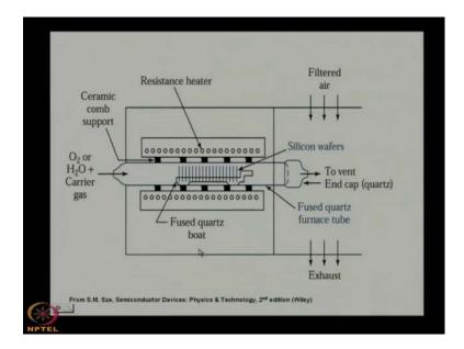
For the oxidation process, we need a reactor and in this view graph you see that this is the oxidation reactor and which consist of these are the parts of the reactor. It consist of a resistance heated furnace this is the resistance heated furnace and this furnace can be resistance heated it can be inductance heated it can be lamp heating like quartz lamp etcetera.
