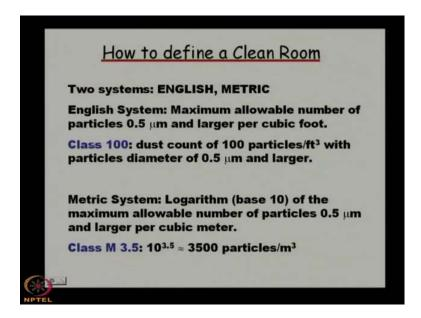
It can be class 100, it can be class m 3.5, it can be class 10, it can be class 1000 and we shall discuss those thing. Practically, a dust particle incorporated into the gate oxide can result in enhanced conductivity and cause device failure due to low breakdown voltage suppose we want to make a MOS device.
