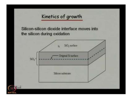
Now, when we talk about the growth of the of oxide layers, so let us talk about the kinetics of growth what is kinetics of growth how the oxidation takes place though oxidation takes place.
