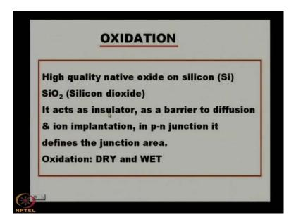
So, from our discussion it is apparent that the oxidation is very important process technology and you see that the high quality native oxide on silicon. The term is very important here is the native oxide which is not, which is not available in except for the silicon in whole semiconductor family.
