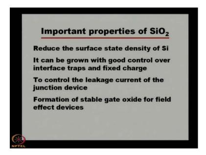
It reduce the surface states density of silicon as we have mentioned earlier that basically the surface state density originating from the unsaturated covalent bonds or the dangling bonds because of the cut of the slice from the mother ingot. That we have discussed earlier that the whole crystal is obtained as the bulk crystal which is say 4 inch, 6 inch, 10 inch or even more than 20 inch diameter.
