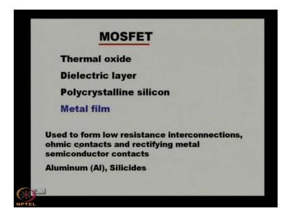
In metal film, it is used to form low resistance interconnections Ohmic contacts and rectifying metal semiconductor contacts and aluminum is widely used in silicon technology. There is lot of research on aluminum and also the silicide like your iron silicide or titanium silicide or aluminum silicide a large number of silicide is also used for the metal film.
