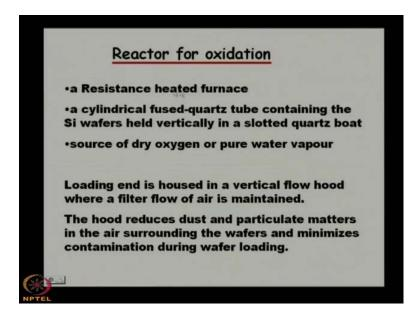
So, this is the figure, it is the resistance heated furnace, then a cylindrical fused quartz tube containing the silicon wafers held vertically in a slotted quartz boat. So, a cylindrical fused quartz, this is the cylindrical fused quartz and this is the slotted quartz boat on which the
