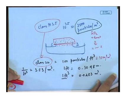
Suppose, we have the class m 3.5, so what is the value of class m 3.5 say class m 3.5 means ten to the power 3.5 and approximately it becomes 3,500 particles per cubic meter approximately the value is say 3 2 0 0 or such. Let us take as 3500 into 10 to the power 3.5, these particles per meter cube, now class 100 it is basically 100 particles per cubic feet. Now, we know that one foot is equals to 0.3048 meter, now if you take one feet cube then it becomes 0.0283 meter cube.
