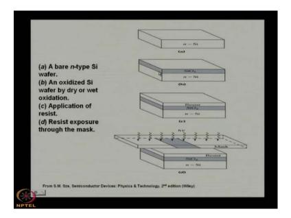
Then, if you find that for the formation of a p n junction, you see that if we start from an n type silicon wafer. First is to grow a layer of silicon dioxide on it, so this is the first step which defines the p n junction, so oxidation is very important step for this processing.
