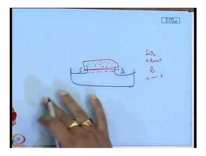
We have gate oxide, this is the substrate then this is the source then this is the drain and this is the gate this gate a channel must be formed just below the gate oxide and this gate oxide must be an insulating one. Now, if there is a particulate or some dust inside the oxide inside the insulating material, then what will happen? Suppose Si O 2 we would like to grow it is insulator and almost 11 is the dielectric constant and if we add some dust with it may be that 11 will reduce to 2 or 3.
