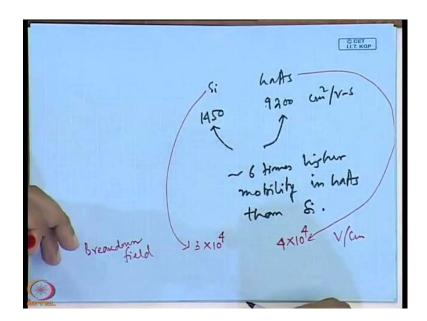
The mobility for gallium arsenide is 9,200 centimeter square per volt second if we compare with silicon which is 1450. So, if we compare this 1450 with 9200, we will find that it all almost 6 times higher mobility in gallium arsenide than silicon. So, the mobility is very high and also the breakdown field which is in case of silicon is 3 into 10 to the power 4 in comparison to 5, 4 into 10 to the power 4 volt per centimeter.
