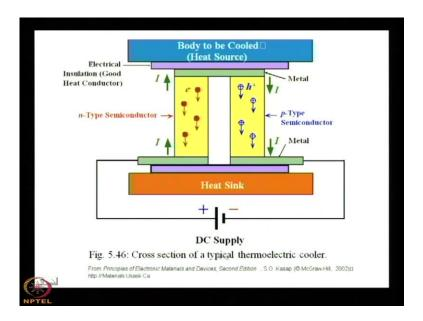
And with this arrangement you see that this is a thermoelectric cooler, where the body to be cooled is placed on the cold junction, this junctions are cold this is an n type semiconductor this is a p type semiconductor. And in a n type semiconductor this junction is cold for a p type semiconductor, this junction is cold so this has been connected to some copper wire say it is a metal means, it is copper then electrical insulation is there.
