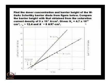
This one, find the donor concentration and barrier height of the tungsten gallium arsenide Schottky barrier diode from figure below. Compare the barrier height with that obtained from the saturation current density of this. Given this N c equals to 4.7 into 10 to the power 17 per centimetre cube. Epsilon s equals to 12.4 and effective Richardson constant A star equals to 8 ampere per Kelvin square centimetre square.
