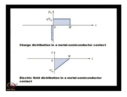
Now, if you consider this thing here, you see that this is the n type semiconductor. This is the metal. The metal is very heavily doped compared to semiconductor n because the number of free electrons in the metal is very, very high compared to the semiconductor not heavily doped. The term doping is not applicable for metal. The exact term should be the number of free electrons on the metal site is more than the number of free electrons on the semiconductor side.
