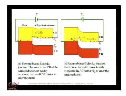
If you see this view graph that means this is the positive potential, which is being subtracted from the built in potential. That means on application or positive voltage, it is reducing. On application of reverse voltage, it is increasing.
