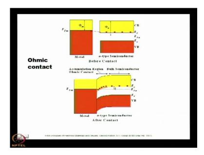
This is because the value of E c minus E f will be less. If the value is sufficiently high, then it can even go upwards. Here, you see that the band bending was such that it even
