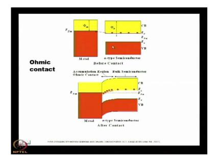
See here; the metal work function is less than the semiconductor work function. It is n type semiconductor. The metal work function is less than the semiconductor work function. Then, if you join, what will happen? Electrons are coming from metal (( )).
