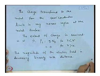
So, the charge transferred to the metal, the charge transferred to the metal from the semiconductor limits in very narrow n region very narrow region at the metal surface. The extent of charge in semiconductor is w that is rho s is equals to q into N D for x less than w and that is equals to 0 for x greater than w. That we have seen in the, we have shown in the graph also the magnitude of the electric field is decreasing linearly with distance.
