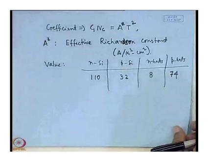
c 1 N c is known as A star T square, where A star is known as the effective Richardson constant, effective Richardson constant. Its unit is ampere per Kelvin square centimetre square. The unit of Richardson constant depends on the effective mass. What is the value of this A star? Value of a star is value 4 phi.
