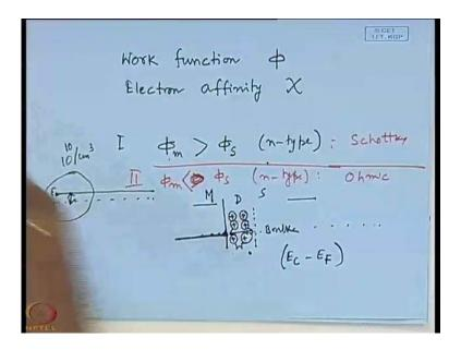
So, that means if we start from this thing that; here, you see that we have started with this slide that phi m greater that phi s for n type, we see that it is Schottky; and number 2 case is that phi m greater than phi s for n type and it becomes ohmic. So, you expect that
