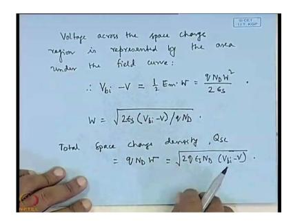
Now, voltage across the space charge by the area under the curve voltage across the space charge region is represented by the area under the field curve. Now, what is the area half base into altitude half base is w altitude is E m. So, that means it is equals to half of E m into w. Now, if you put the value of E m, you will get q N D w square by twice epsilon s. So, that is V b i minus V. That means some forward bias we have applied.
