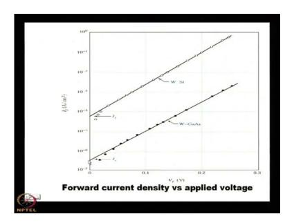
It is forward biasing. You would see for 2 cases. One is silicon on silicon where tungsten is, tungsten contact is made here. The same tungsten constant contact is made on gallium arsenide. You see that it is seen by this arrow. The value of the J s, the J s can be measured from the extrapolating the J v curve to V equals to 0. This axis V is on this axis. V is 0. So, extrapolating this curve to V axis will give you the value of J s. Once you know the J s, you can calculate the barrier height.
