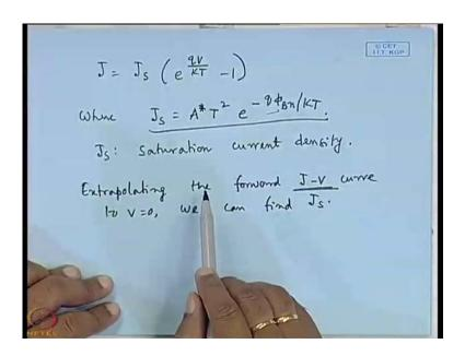
If I write down the net current, I can consider this to be J s or the saturation current. This is J s, which is not the saturation current. So, net current J can be equals to J s e to the power q V by K T minus 1 where J s is equals to A star t square e to the power minus q phi B n by K T. J s is known as saturation current density.
