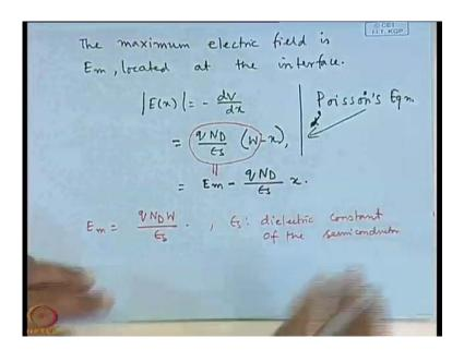
The maximum electric field is E m, located at the interface. Maximum electric field is located on the interface. Now, you know that the electric field is given by minus d V d x. That is equal to q N D by epsilon s w minus x. From does it come? It comes from the Poisson's equation. That equation is basically related to the electric field and the, or the potential and the charges potential and the charges the relation between the potential and the charges.
