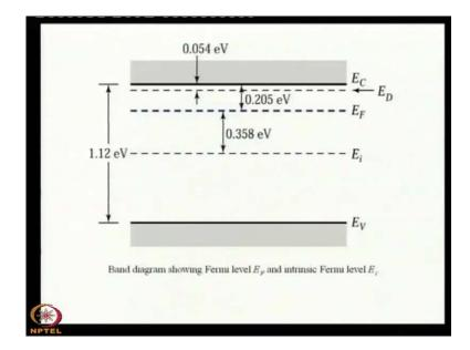
But you see here. This is a diagram where you see that E D is shown; this E D dotted line and what is this E D? E D you see that 0.054 electron volt, below the bottom of the conduction band; E C is the bottom of the conduction band or the conduction band minimum. 0.054 electron volt is the value just below the conduction band, there is a donor level or defect level.
