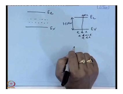
So, though ideally there should not be any electronic or hole levels in the forbidden gap. There may be some levels due to impurity or vacancy or defect and this thing was discussed; that it can be intentionally or unintentionally, intentional levels are basically
