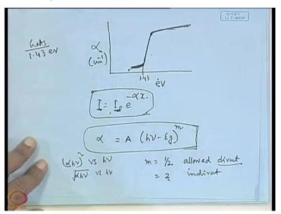
When aim is half then direct gap then alpha h nu square is plotted as a function of h nu. But when it is 2 for indirect band gap semiconductor then it is alpha h nu root over of versus h nu is plotted. And, the same technique is adopted that the linear portion when extrapolated in the energy axis will give you the band gap. So, that is very easily you can calculate the band gap of the semiconductor using absorption spectroscopy where it is not a destructive technique.
