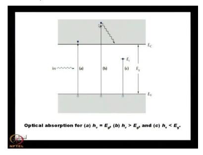
Now, if we see this view graph, you see in this view graph the as soon as you excite the electrons with some energy there may be different situations. Here, I have seen you the three situations. In situation a it is band to band transition that means the energy is basically equal to band gap energy.
