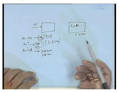
In photo luminescence what actually is done? The sample is excited by means of a optical source. Generally, the optical source is a laser source generally. So, that means what kind of laser you can expect? It must be greater than the band gap energy of the material otherwise the laser will not be able to excite. So, chose that laser in that manner. Suppose your material is zinc oxide. What is its band gap what is the band gap of zinc oxide?
