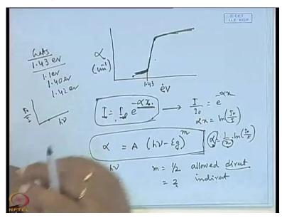
So, basically it is I0 by I which is basically plotted. And, from that plot you have to measure alpha h nu square versus h nu. That means you need the thickness because you need the thickness; x is the thickness. Unless you know the thickness you cannot measure alpha h nu square versus h nu. So, thickness is important. Then how you will determine alpha? From this equation how you determine the alpha?
