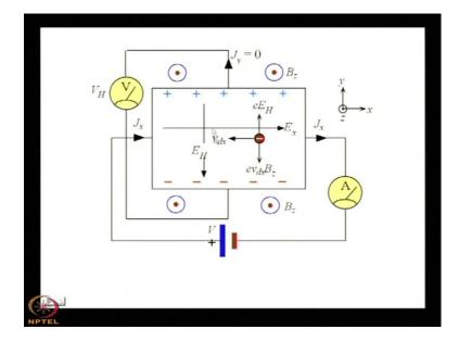
Now you see that suppose you have this type of a semiconducting bar or let us consider that this is the metal bar. Let us consider that this is a metal bar; forget about semiconductor in the first case. The current passes through this x direction, positive x direction it is say; it is the positive x direction and the magnetic field is in the which direction? z direction.
