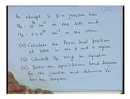
Now let us quickly have a numerical problem an abrupt silicon p-n junction has N a equals to 10 to the power 18 centimetre cube inverse on one side and N d equals to 5 into 10 to the power 15 centimetre cube inverse on the other. a) Calculate the Fermi level positions at 300 Kelvin in the p and n regions; b) Calculate V b i using an equation and c) Draw an equilibrium band diagram, draw an equilibrium band diagram for the junction and determine V b i from the diagram.
