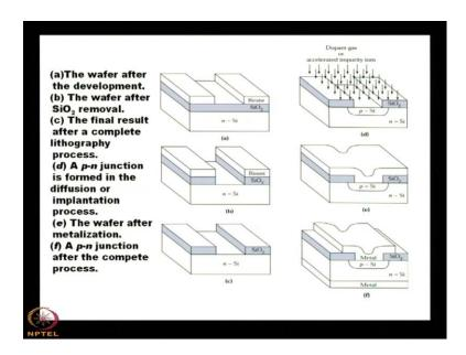
So this is in the next, in this diagram you see that, here this is that region where this is the photo resist coated area and the wafer after the development will look like this. Development means, since ultraviolet light was used; so it is exposed. So, you put the sample in a developer. It is like photography you put it in a developer, so these portion will go out; right.
