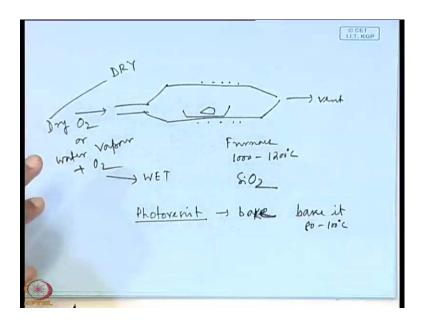
This is the furnace. This is the quad's boat on which the silicon is placed. Then, this is the vent through which the byproducts will leave from the furnace. This is the temperature heating element which can be control and you send either dry oxygen or water vapor plus oxygen. For dry oxygen, it will be dry oxidation; it is it will be wet oxidation.
