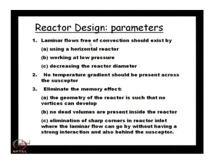
So, in a sense we can say that laminar flows free of convection should exist by using a horizontal reactor working at low pressure and decreasing the reactor diameter. So, a decreasing the reactor diameter how you decrease the reactor diameter the reactor diameter can be decreased if you make the susceptor inclined to make the susceptor inclined then what effectively the diameter reduces it is like this.
