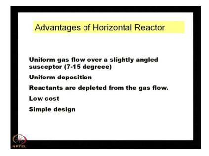
It is a horizontal reactor what are the advantages of horizontal reactor the advantages of horizontal reactor is that uniform gas flow over a slightly angled acceptor this is 7 to 15 degree because it has been proofed that the gas flow will be uniform. If there is a certain slanting of the susceptor because of the velocity problem that we shall come uniform deposition reactants are depleted from the gas flow low cost simple design.
