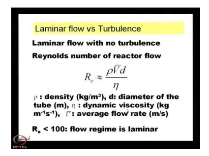
Now, very important aspect is that for very good CVD reactor we have to consider two important aspect one is that the gas flow must be laminar flow not turbulent the opposite of laminar is turbulent you know what is turbulence that is random.
