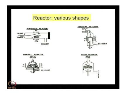
There can be say, it can be atmospheric pressure CVD, it can be low pressure CVD, it can be p type CVD, plasma enhanced CVD. There is one type of CVD which is known as the metal organic chemical vapour deposition, as the name implies there we use the metal organic as the precursors. Now, what is the advantage of metal organic precursors the advantage of metal-organic precursor is that it can be volatile.
