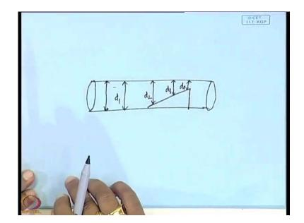
This is the uniform tube or reactor you want to make the diameter less the effective diameter becomes less effective diameter becomes less because here the diameter is say d 1 here, it is d 2 here, it is d 3 here, it is d 4. So, the design principle is based on those facts that you use a horizontal reactor you use low pressure and decrease the reactor diameter. Then, you can ensure laminar flows free of convection sir which diameter we will take in that case which diameter in the in the reactor.
