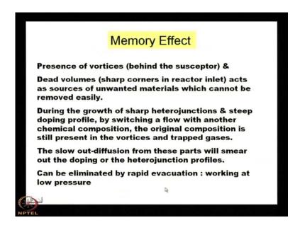
Now, what is memory effect, memory effect that is behind the susceptor and sharp corner in the reactor inlet. There may be unwanted materials yes you see that when it is placed when it is placed there is dead volume behind this susceptor because gas is coming out from here. So, gas is filling the whole volume of the reactor reaction taking place on the front side where there is a temperature hot zone.
