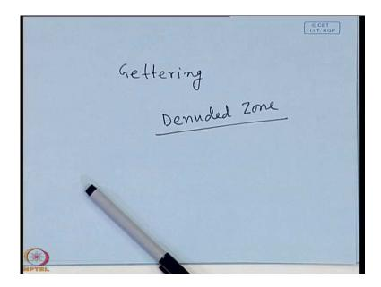
There is one term in crystal growth which is known as Gettering, which is known as Gettering. Gettering is a process which removes the unwanted impurity from the surface to the bulk from the surface to the bulk, that is known as Gettering.
