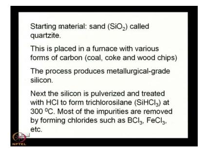
So almost all of the silica materials; which are used as the starting material for silicon crystal growth come from the Brazil or China. Then this silica is placed in a furnace, starting material is sand called quartzite, this is placed in a furnace with various forms of
