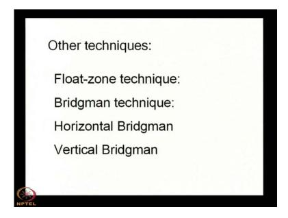
So, those are the reasons that single crystals material are grown. There are other techniques also for crystal growth, one is say Float-zone technique another is say the Bridgman technique. The Bridgman technique can be Horizontal Bridgman, it can be Vertical Bridgman and we shall see that for gallium arsenide fabrication this Bridgman technique is used and Czochralski and Float-zone techniques are used for silicon technology.
