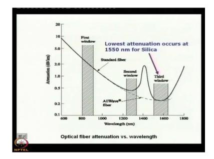
Now, if I see you if I show you this graph. What is there? You see that it is in the y axis I have plotted the attenuation in decibel per kilometre and in the x axis I have plotted the wavelength in nanometer. So, it is a attenuation versus wavelength curve, it is a attenuation versus wavelength curve.
