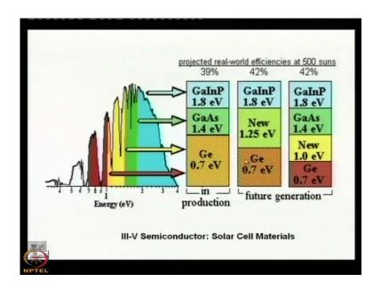
So, many materials are involved you see that in this view graph I have plotted the 3 5 semiconductor energy versus intensity, the left one - this one is basically the solar spectrum which I have shown in the previous view graph. And this is germanium, gallium arsenide indium gallium phosphide, you see that the band gaps are given here, it is 0.7 not exactly point (( )) 0.67 then gallium arsenide 1.43, then indium gallium phosphide is 1.78 electron volt.
