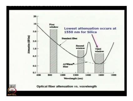
So, let me write down the windows. First window, second window, and third window; for first window it is around 800 nanometer, say it is 850 nanometer. And in micron what is the value 0.85 micron 850 nanometer means 0.85micron; that means, 8500 angstrom. Second window it is 1300 nanometer and the third window is 1550 nanometer right.
