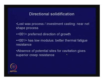
But, this directional solidification quick look, I mean, this I am just named, so this is the, because they cannot be deformed. So, the material, when you make the product it should be near net shape product and this is done by precision casting and lost wax process and investment casting. These are the techniques, this is the cube, direction is the preferred direction of growth, this is the direction, growth rate is maximum and often, this is also direction, which has low modulus.
