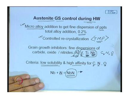
Andhow do you do it and this is what we will cover in the next fewslides. Now, how do you control this austenite grain size control during hot working? Now, this is where you can make some micro alloy additions say normal, if it is iron carbide it dissolves at a quite a low temperature therefore, this iron carbide or cementoid is not very effective in controlling or in suppressing the growth of austenitic grain.
