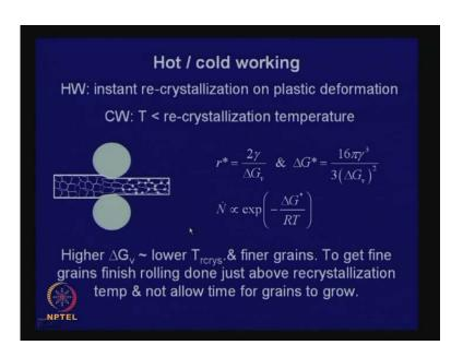
And if you recollect yourlastlecture, we talked about thermo mechanical processing. If the working is done above re-crystallization temperature, we shared it is hot working and the bulk of the deformation from the continuously cast (()) is done through hot working. And cold working is often done in the finishing stage and often after cold working the steel may have to be given some amount of annealing to relieve the stresses or to get
