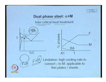
Now, a quick look at this we looked atby thermomechanical processing by controlling the transformations, how we can get how we can get extremely fine grain structure, and which have and which have very good strength and toughness and as we will see later they also have very good weldability. Another important class of steel where you get good combination of strength and ductility is the dual phase steel.
