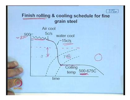
In arolling millwhich is schematically shown over here, finish rolling which is done over here. And this finish rolling temperature is substantially low that is, may be depending on that carbonconcentration, it could be around 850 to 900 degree centigrade you finish the rolling. And after that here the rolling is over, and then you cool it little rapidly, so that you cool it little rapidly this temperature cooling it rapidly.
