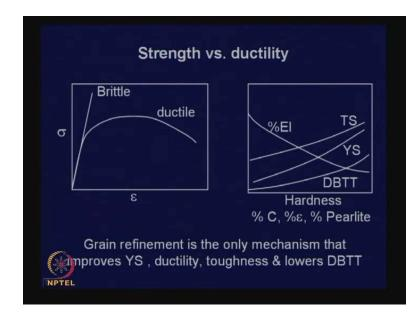
Now, by most of these strengthening mechanisms if you try to increase the strength of crystal, what happens? What effect does it have on the ductility? If you recall it out that
