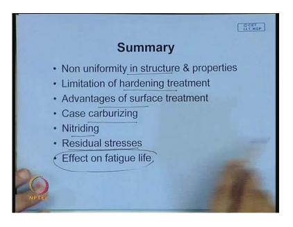
So, therefore to sum up what we have looked; at we looked at the non uniformity of structure, and uniformity structure properties, limitations of hardening treatment, advantages of surface hardening, we talked about case carburizing, nitriding, origin of residual stresses and its effect on extending fatigue life. Thank you very much.
