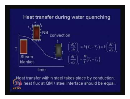
Now a quick look at the heat transfer process of heat transfer when you quench and let us see, look at it little more critically say here if you quench, this is a section of a job, which has been quenched in water. When you quench it has a very high content of heat so suddenly what happens, a blanket – a steam blanket will form over here. And when a blanket - steam blanket this has a relatively low conductivity and it is stagnant, so you have a poor heat transfer coefficient.
