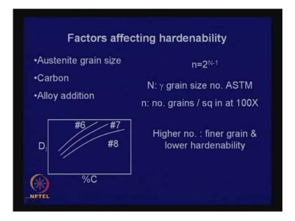
And let us now look at the factors that affect hardenability part of it was explained last class, and there are primarily three main factors which determine hardenability one is austenite grain size and we talked about determining austenite grain size ASTM method is like this. And n is the number of grains you see at 100 magnification at 100 X and n represents number of grains in one square range, and this is n is an index which is a number.
