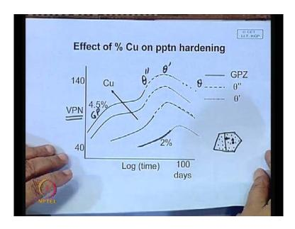
Now, when this process of precipitation takes place you have different types of precipitate forming in the matrix, and obviously when this precipitate form in the matrix what it will do, it will make, it would process of deformation more difficult because we have learnt that metals deform by movement of dislocation. So, this precipitate gives in the matrix, if you have the matrix, you have precipitate the dislocation which is there. It will be difficult for it to move or cross this precipitate.
