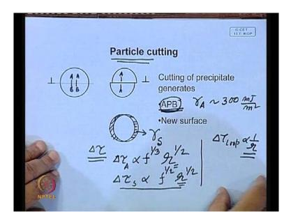
In the same way it is possible to do similar calculation for particle cutting. You go into the detail of the process of calculation, but here two things happen. When the precipitate is sheared, here if there is a, this is a order precipitate. so you have bond A B type bond here, here you see, here you see, so if you slip it, you may find say then, if you slip it, you may find this, is a this also becomes.
