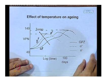
So, that means the extent of hardening will depend on the chemical composition that alloy content and as well as it will also depend on the time of ageing. It will also depend on the temperature of ageing so if you age at a higher temperature you have less number of precipitates, you know. Say, suppose if the highest temperature over here which is shown then there is no chance of G P zone formation. G P formation takes place at a lower temperature its (()).
