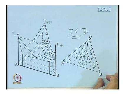
And here is the horizontal section at a temperature below the eutectic temperature. So, that means this horizontal section is below the ternary eutectic; let us say at room temperature. This is the alpha end; this is the beta; this is gamma; this is alpha plus gamma; this is alpha plus beta; this is gamma plus beta. And in this region, you have the eutectic; that is ternary eutectic will be there in this region; alpha beta gamma. This portion you will get binary eutectic alpha gamma, gamma beta.
