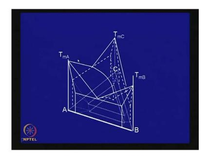
Now, let us look at this diagram the nature of this diagram, which is... Here these are the three axis; here you look at this is the liquidus surface, which is coming down from that melting point. Say on this line is the T m A is the melting point of A. This is the liquidus surface; this line similarly consisting of this.
