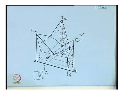
So, in this if you look at here this line, this surface, this, this; then this line, this surface; this is one phase; liquidus phase. Similarly, there will be one consisting of this, this and then this, then this, this. Similarly, a third surface will be from a melting point of B and
