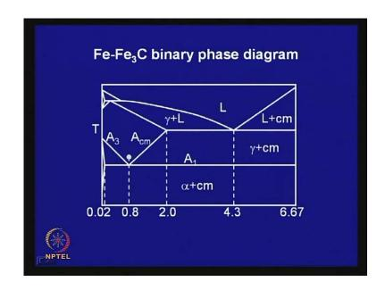
Now, let us look at the structure of this eutectoid steel critically. Last class, we looked at that if you cool a steel from this austenitic region, which has a carbon content which corresponds around 0.8. So, this is the eutectoid point. What happens as you cool at this eutectoid temperature around 723? As you go below the 723 degree centigrade, you have precipitate; I mean this austenite breaks down simultaneously into a fine mixture of ferrite and cementite and this is called pearlite.
