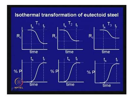
Say, you prepare a table or you make a plot let us say. If you make a plot say first how does at a particular temperature? Say, suppose this is the intermediate bath has temperature T 1 and in that case what we have seen? The first sample when you quench after certain time, you get the maximum hardness and this is around 64. Say, this is what we have seen.
