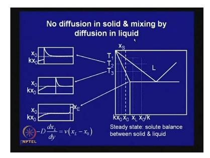
Now, let us move on to a case where there is no diffusion in solid; but there is mixing by diffusion in liquid. In this case the few cases, which have been represented here. Let us consider the similar system exactly here. Say, suppose at this temperature say T 2
