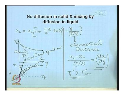
So, that means and if you try and plot; that means the concentration in the liquid will be equal to x naught 1 minus then an exponential term minus this is the distance over D minus v. Now, here look at this dimension. This dimension of this is also that of a distance and this is called a characteristic distance characteristic distance for the concentration profile. So, that means from that interface, say suppose this is the interface and here your concentration at the interface is x L.
