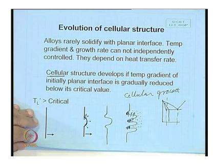
Let us case; but in reality if you look at alloy system, the alloy they rarely solidify with planar interface. And the temperature gradient and growth rate; they cannot be independently controlled often and they dependent on heat transfer rate. Now, let us take up a case and see, when cellular structure develops; we will come to know what is cellular structure. Now, suppose if the temperature gradient is initially favours planar
