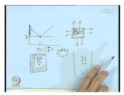
Now, water actually has dissolved gas; that means air is dissolved in water. And air and water, it forms some kind of a eutectic phase diagram. So, let us assume that water this is pure; eutectic temperature is this; this is the eutectic composition. So, the first that ice
