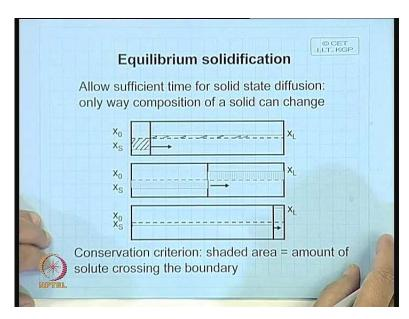
And this is the amount of solute from liquid is getting transferred in to solid. So, this area will be equal to this. So, intermediate stage here also; this area is equal to this and ultimately, when the solidification is above to be completed, the composition of solid you know it comes; it starts here; it moves up; here it moves (()) for the... And ultimately, when it is totally solidified, here will be uniform composition through and through.
