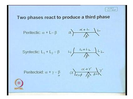
Now, next is the second case, where two phases react to produce a third phase. We looked at peritectic, where alpha reacts with liquid giving you beta, which is shown over here. Now, there are several variants of this, and which, from which you can derive in the same way as that from the eutectic reaction. And here, say like in this particular case,
