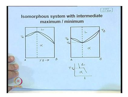
Now, there are cases where this type of isomorphous system can exhibit maxima or minima; so that means, in between an alloy, there can be an alloy, which has in this particular case, higher melting point than both A and B; and which is shown in this diagram. And we will look at it here, say suppose this is actually T over A, this is B, you have percentage of B with percentage plotted along this axis, this is melting point of A,
