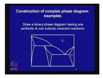
And which is shown here; in this particular case, if you this is pure A, this is pure B, this is liquid, this is one terminal solid solution alpha; and here alpha, this is a peritectic reaction, alpha reacts with liquid giving you an intermediate solid solution gamma; and this is a terminal solid solution beta, and you have an eutectic reaction, isotherm over here.
