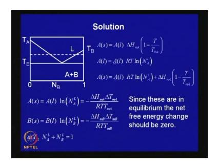
In this particular case, you can see that atom fraction, the large atom fraction A in liquid will be a function of which is shown over here. So, this you can just algebraic simplification, this is equal to this; and you can apply the same concept to this region of the diagram, and then you get similar expression for this. Now, if here, so all these are known, this is known, this is known, this is known, temperature is fixed. So, it is possible
