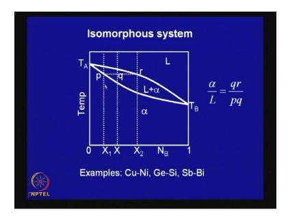
First start with this isomorphous system in the phase diagram, you know just to recollect that, this is that phase diagram of an isomorphous system. And in the two phase region,
