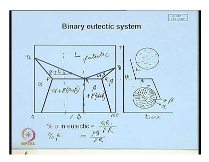
Now, let us look at this diagram once again. So, here this is the percentage beta, percentage B; here this is 0 B; this is 100 percent B. This is the melting point of A; this is melting point of B. And if you can level the diagram here, the phase that is (()) stable
