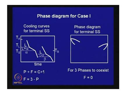
Phase diagram for the case I: Here cooling curve of terminal solid solutions alike this. Now, here you can draw on the phase diagram; here you have temperature on this axis; composition here. Now, take up several alloys; find out liquidus and solidus temperature. And let us consider this A rich portion; here this is the solidus; this is the liquidus. Similarly, terminal solid solution beta; this is the liquidus; this is the solidus. (Refer Slide Time: 08:14)
