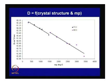
Next, if you calculate diffusivity at say fix temperature possibly I think hundred degrees centigrade and look at this plot. The diffusivity and melting point, so that means if the melting point is higher at a given temperature is diffusivity is lower. So look at this so if
