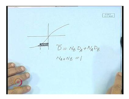
You will recall that inter-diffusion coefficient was derived at N B times diffusivity of A plus N A times diffusivity of B. Now here if we know that N A plus N B equal to 1. So if you substitute this what is the type of variation to you expect? So in this case say suppose diffusivity intrinsic diffusivity D A is over here this is the other one; if you follow this then the inter-diffusion coefficient should be given by this line and which is very evident from look at this expression.
