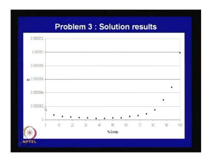
Having done this you try and plot and what you find here is that inter-diffusion coefficient is function of composition. So these are the intrinsic that diffusivity similarly, here also there be intrinsic diffusivity point somewhere here. But in between this inter-diffusion coefficient initially its goes down then again it goes up, so this is interesting look at it.
