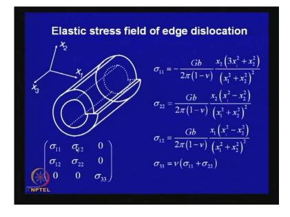
Now, similar calculation it is possible to do for edge dislocation, but edge dislocation, the displacement is, which occurs is little difficult to calculate and you have to have a clear conception of the geometrical distortion that takes place. So, that way we will not go through the total derivation, but we will give you the elastic stress field of the edge dislocation, which is given here. This is how you visualize that.
