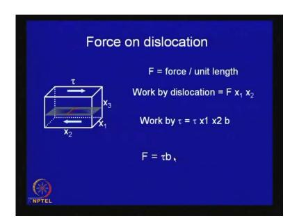
Now, dislocation can move only as a result of applied shear stress and when you apply a shear stress on the crystal on the slip plane, you can imagine, that means, as if the dislocation is there as a line and on that line a force is acting and this force will have a relationship with, have a direct relationship with the applied shear stress.
