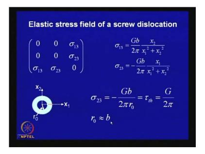
So, what you do here? This gives you the state of stress for around screw dislocations. So, all these components, these are 0 and if you add these, one-third of this is called the hydrostatic stress field. So, which means, that here the hydrostatic stress field is 0. So, this also explains why the vacancies do not interact with screw dislocation because if you create a lattice vacancy around the vacancy, there is a volume change and here you see that there is no volume change here.
