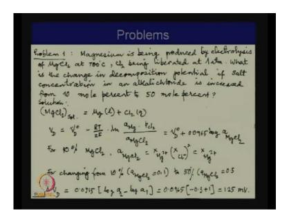
Let us end this lecture with one or two very simple problems that will make use of some principles we have discussed. Here is a problem that magnesium is being produced by electrolysis of magnesium chloride at 700 degrees, chlorine being liberated at one atmosphere. What is the change in decomposition potential, if salt concentration in a alkali chloride is increased from 10 mole percent to 50 mole percent.
