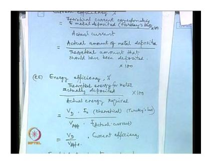
Now we must, when we discuss electro metallurgy define some terms and you should know exactly what they mean, very often we talk about current efficiency, during electrolysis by the word, current efficiency mean, we mean theoretical current corresponding to the amount of metal deposited, you know you have during electrolysis produce certain amount of metal.
