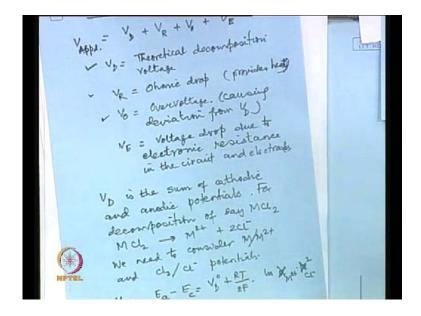
The expression is applied voltage is sum total of four terms first of course, is a theoretical decomposition voltage, which you must exceed to decompose the metal then there is a ohmic drop. There is a resistance in the bath, which because of which there is a voltage drop called V sub R, then there is that over voltage phenomena.
