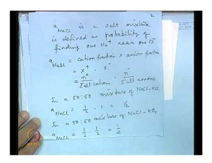
X cation, X anion, which will be represented by number of cations in the entire mixture divided by all cations in the mixture, because this ratio will give us the probability of finding a cation in the cation sub-lattice. And at that point, n minus 1 by all n anions will give us the probability of finding an anion in the anion sub-lattice and the product means that there will be together, so that gives us the probability.
