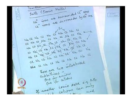
The Temkin Model for Fused Salts or Ionic Melts says that in the ionic media, there are two sub-lattices: one sublattice for the cations, one sublattice for the anions.
