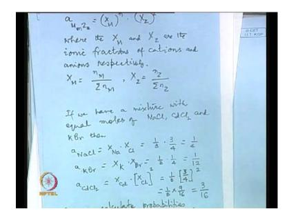
Now, the generalized expression for activity of a salt M sub m, Z sub z, dissolved in an ideal fused salt mixture is given by activity term, ionic fraction of M to the power m, ionic fraction of Z to the power z, where X sub M and X sub Z are the ionic fractions of cations and anions respectively, this is the definition of the anion fractions.
