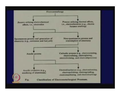
Let us look at the way Electrometallurgy is classified. Electrometallurgy can mean processes using electrochemical effects that necessarily make use of electrodes and that
