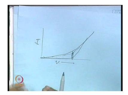
Now, in much system there is a very simple method of finding out what is the voltage required for electrolysis and that is that we will pass through two electrodes, a current and will plot, will apply voltage and gradually increase the voltage and see the current passing through the medium.
