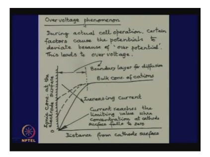
The explanation to this phenomena rise in what we called, the over voltage phenomenon over voltage phenomenon is the phenomenon which changes the normal zinc, zinc ion potential. Means the electrode potential will no longer be what you have seen in the electrode potential series.
