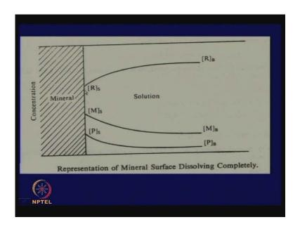
Now, considered basically what happens in a leaching reaction, we have a mineral surface, it is not a pure mineral it may have other things also, but the idea is that a reagent has to come to the mineral surface, react, produce a metal ion or a metal ion complex which will be taken into the solution, this is the metallic value we get. And when this is reacting with the regent that has come to the mineral surface, you may produce some other products which will diffuse out entity bulk.
