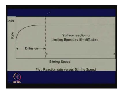
Now, here is a situation where a reagent is going from the bulk to the surface, now this is where actually the diffusion is taking place, diffusion in the boundary layer is taking place, because it is been eaten up here the species has to move toward this, and then from here to here it goes because there is a concentration gradient, this minus this divided by a boundary layer, diffusion layer and that defines a boundary layer.
