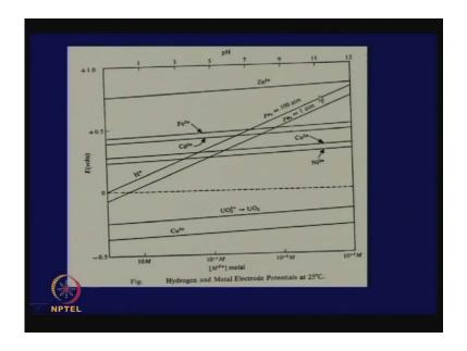
So, here is a simple diagram to explain this, we are plotting here the electrode potentials of copper, iron, cadmium, zinc, nickel, cobalt. In this axis we are putting metal ion concentration in molal. Here there is a p h axis for hydrogen, this is the potential. The plot gives us... these are the plots for hydrogen, by increasing the pressure from 1to 100 atmospheres there is only change this much of change. Whereas, these are the lines for
