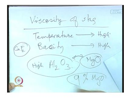
So the viscosity of slag which is a crucial parameter in pyrometallurgical operations depends on temperature because, the higher the temperature lower will be the viscosity no matter what slag is it because, at higher temperatures bond strength to break and the other will be basicity. So temperature should be high basicity; should be high to lower viscosity or increase fluidity. There also some fluidizing agents like calcium fluoride which when added increases fluidity of slag.
