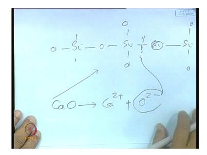
And this is, if let us represent the basic silica structure by two dimension in two dimension; these are oxygen atoms. If we add to this silica which is an acid oxide a basic oxide like calcium oxide which gives calcium, this oxygen goes and breaks a silicon oxygen bond so it splits, we from a big flow unit, we create two smaller flow units and then, it becomes less viscous.
