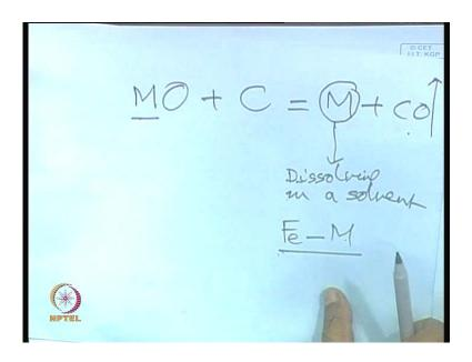
That suppose, there is a metal oxide which is reduced by carbon to form metal and carbon monoxide.
