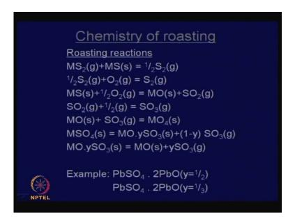
Let us now proceed. The thermodynamics has been extensively applied in the case of roasting reactions also to understand the reactions. Now, during roasting all kinds of
