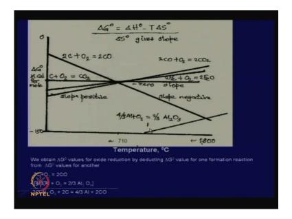
Now, let us take this example of reduction of Al 2 O 3 by carbon. So, we have to combine these two reactions; 2C plus O 2 2CO and 4 by 3 aluminum plus O 2 2 by 3 Al 2 O 3, you have to deduct the free energy values for this reaction from the free energy change for the axis reaction and then, we get the desired reaction 2 by 3 Al 2 O 3 plus 2C
