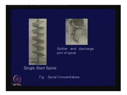
And how does it function? We have shown you a picture, a slurry will come down from the top, it will come at increasing velocity, rotating and during the process of rotation, the particles minerals will get separated depending on their density,
