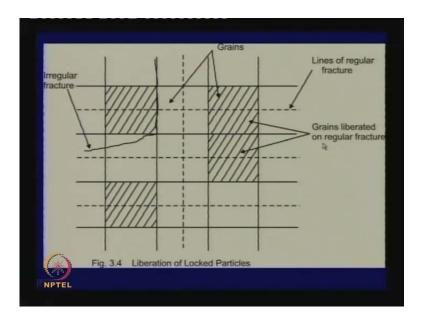
This is regarding how particles fracture, they can fracture around the grains, they can fracture across the grains. Then, I have talked about what kind of particle size that different particles have.
