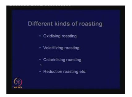
Now, there are many, many steps in any roasting operation, oxidizing first is roasting. You roast. In roasting there is necessarily release of some gaseous substances oxidizing. Roasting means you change, say carbonate into an oxide. Volatilizing roasting means you take out some volatiles. Caloridising roasting means you make a chloride reduction. Roasting means you reduce.
