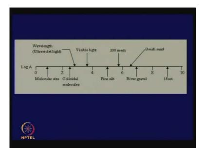
To give you an example, why, what happens in a size reduction, here is a simple to give you an idea as to what we mean by size reduction. This is a typical size ranges for various materials, it is in angstrom unit.
