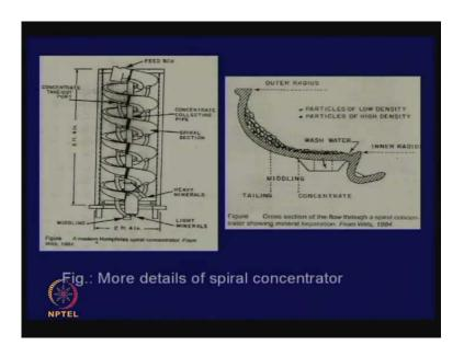
When that is happening if you see, it is a trough which goes with a slope downwards. How will the water flow in water? We will have 0 velocity in contact with the perimeter, it will have a 0 velocity at the center, so there is a velocity gradient from the center to the side at any place, at any place here from center to the perimeter, there is a velocity gradient.
