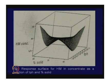
Well, this can be done put in terms of the computer camera also, print that for heavy metal in this case, it is heavy heavy mineral, it can be for very heavy minerals all together or single minerals, we can plot them heavy mineral in the concentrate as a function of percentage solid and tonnage per hour, we did something like that for very heavy minerals also.
