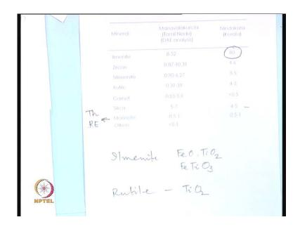
Now, in the beach sands in the Tamilnadu coast, this is an analysis given in one source, it may contain from 8 to 52 percent ilmenite, zircon 0.87 to 10, sillimanite, rutile is T i o 2, then garnet, silica, monazite this is important, this is important because it is a source of thorium and rare earths and there are some others.
