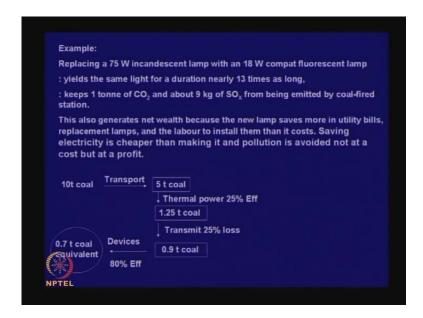
Replacing a 75 watt incandescent lamp with an 18 watt compact fluorescent lamp yields the same light for duration nearly 13 times as long it keeps one turn of CO 2 and about 9 kg of SO x from being emitted by coal-fired station because it is consuming less electricity.
