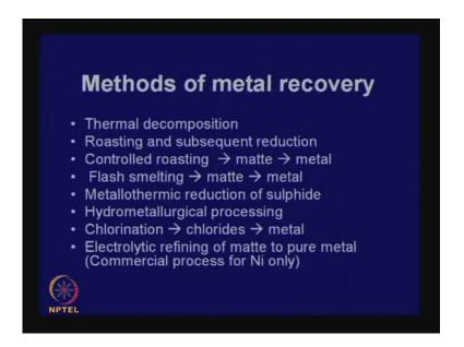
Now, these are the standard methods of producing metal from sulphides. One is straightforward; it is 'Thermal Decomposition'. This is applicable in the case of mercury sulphide: Hg S, which can be simply heated and it decomposes to give mercury metal and sulphur. Most common and logical will be to take the sulphide, roast it to make an oxide, and then reduce by carbon, like the way you treat an oxide.
