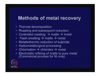
Flash smelting is an improved step, improved process of combining roasting and matte smelting. Then if we can produce a pure metal sulphide, you can always go for metallothermic reduction also, because there are some metals like calcium which can produce very stable sulphide and so these base metal sulphides can be reduced.
