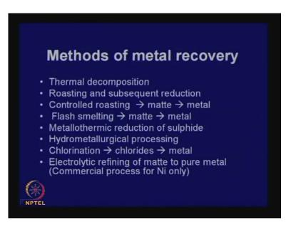
Now, before I proceed further, you should know, what are the general methods of getting metal from a metal sulphide? There are some very standard approaches. One is thermal decomposition. There are many sulphides which simply decompose on heating; example is mercury sulphide, Hg S.
