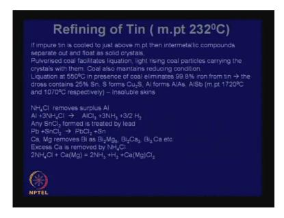
Now, this you should understand. If impure tin is cooled to just above the melting point then many intermediate intermetallic compounds that exist as impurities, will separate out and float as solid crystals.
