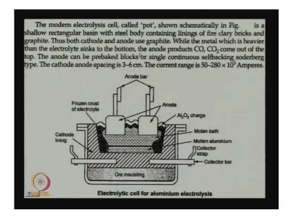
Three to six centimeter, is the inter electrode separation. Both cathode and anode use graphite, the metal is heavier than the electrolyte sinks to the bottom, the anode product CO, CO 2 to come out of the top. Anode can be prebaked blocks or single continuous Soderberg type electrodes. Spacing is three to six, and it has to be maintained, as consistent as possible and of course, the current range can vary a bit. Well that is all, I would say about aluminum electrolysis for now.
