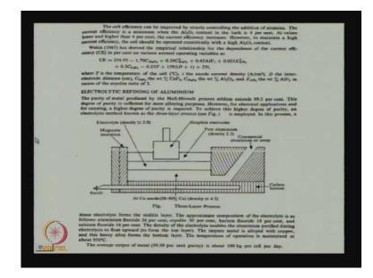
Here is the scheme, the purity of metal produced by a Hall Heroult process is 99.5 percent. Now, this purity, is sufficient for most alloying purposes, but for electrical applications, and for canning, which requires lot more improvement of mechanical properties; formability, one needs a higher purity, and to achieve this higher degree of purity, there is an electrical electrolytic method, call the three layer process.
