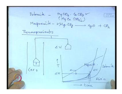
So, reduction is driven to the right by vacuum condensation of magnesium vapours and that will eliminate back reaction also. Now, before I proceed with this, let me ask you simple question. We are talking about two main things - one is dolomite which is MgCO 3 CaCO 3 or you can write it as MgCa CO 3 twice or we are talking about magnesite MgCO 3. How do you know at what temperature it will decompose? There is a very simple way of finding that in the laboratory. That is why thermogravimetry.
