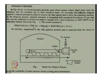
We have just consider one reaction and calculated the partial pressure of magnesium and we have come to the conclusion that it has to be less than 15 millimeter MgO. This is exactly what was done, what was accomplished by gentlemen called pidgeon with some of his associates during the Second World War.
