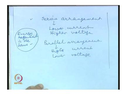
So, you have a choice between a series arrangement where we have lower current because the same current is flowing through but higher voltage. The voltage is adds up or you can have a parallel arrangements where we have higher current, because the current will get split into different things but you will have a lower voltage, because from two common grids, all of them can be operated. Now, question is this better or is this better?
