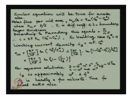
Now, the similar equation will be true for anode also. Now, molar flux per unit area is total flux divided by a which is the a constant into c naught minus c s naught; c naught is the bulk concentration and c s is surface concentration is the diffusion coefficient, and where a k m is d by delta; d is the diffusion coefficient and delta is the boundary layer thickness. You know, you know, here available diffusion coefficient.
