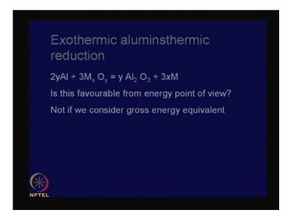
Many oxides, which we have written as MxOy, can be reduced by aluminum, because aluminum forms a more stable oxide Al2O3, and it releases the metal. For example, if you can take Fe2O3 and mix with the aluminum powder, all that one has to do is simply to ignite it, and there are many methods of igniting.
