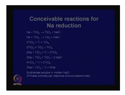
I propose that it does not occur like that. Actually, there are simpler reactions that take place. Like sodium reacts with one molecule of titanium tetrachloride, produces a sub halide such as titanium trichloride, which then dissolves in sodium chloride. Then sodium reacts with titanium trichloride, which is in the liquid state, produces another sub halide titanium dichloride and sodium chloride.
