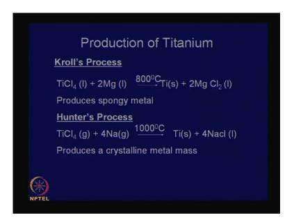
Now, let me give you, write, discuss two equations. To tell you how... that when you write an equation in non-ferrous metallurgy, we are not doing what we do in chemistry. Had this been, a course in chemistry, I would have said that sodium can be titanium can be produced by reduction of titanium tetrachloride by magnesium or reduction of titanium tetrachloride by sodium and period, and then I proceed to something else.
